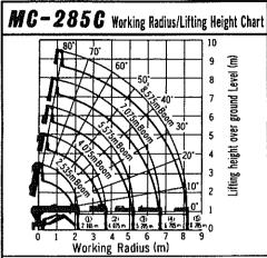
I This chart does not reflect any bending of boom
