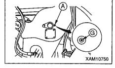
4. Loosen the oil inspection plug © by turning it with the Allen key © to check if gear oil oozes out.
