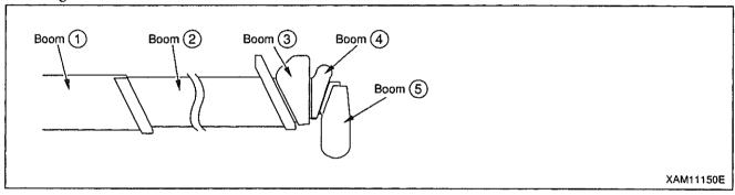
3. "5.575m Boom": Boom extended to such extent that the first mark of the boom 3 is exposed. When the boom 3 is extended by any amount, however, work should be carried out according to the performance shown in this column.
