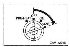
4. When the engine starts, release the key, It will return to ON position automatically.
