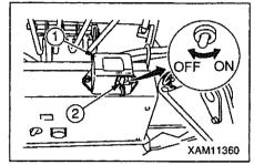
3. Press down the lever 4 of over-hoist alarm system 3 to check that the alarm buzzer stops.
