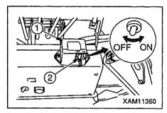
• Over-hoisting the hook block causes the warning buzzer of over-hoist alarm system to sound.
