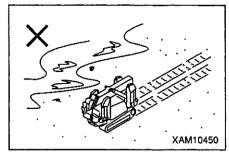
When handling food products such as salt, sugar, wheat or soy beans, if deep scar exists on rubber track, broken pieces of wire or rubber may enter. Correct any damaged rubber portion before use.
