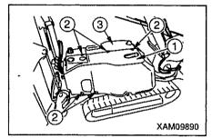
Remove 3 mounting bolts 4 of the right hand side machinery cover
