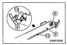
8. Pull out the inner box 10 from top box 9 and align the hole on top box 9 with the position of innermost hole on the inner box 10.
