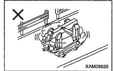
Do not operate the machine to rub rubber track edge against concrete ridge or wall.
