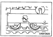
• In case the tension is strong (to reduce tension)
