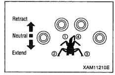
4. After both tracks are completely grounded, continue to push up the outrigger switch, one at a time or 2 simultaneously to IN position. When, with the outrigger telescoping cylinder having retracted completely, the outer box (9) has reached upper limit, take your finger off the outrigger set up switch.
