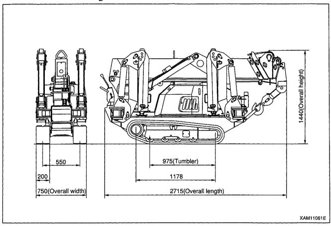
★ The above drawing shows the machine with its travel lever stand in Hauling position
