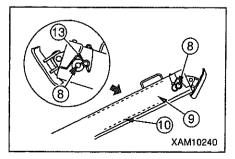
4. After removing the snap pin ② at the end of positioning pin u of linkage bracket ①, pull out the positioning pin ⑦.
