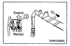
Slowly operate winch lever back and forth to check that hook block is hoisted and lowered smoothly, that it stops immediately when the winch lever is returned to Neutral position and that the winch does not take up the rope in disorderly manner. Correct any abnormality as necessary.
