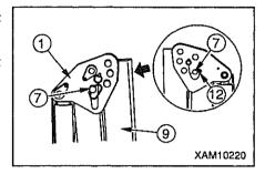
7. Pull out the positioning pin 4 of the rotary 3 and turn the rotary to inside.
