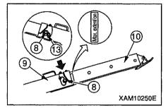
9. Insert the positioning pin (8) to the hole of top box (9) and retain it with the snap pin (13) at its end.
