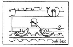
In case the tension is strong (to reduce tension)
