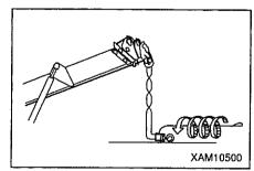
In case the twist can not be removed in spite of above procedure, replace it with new one.
