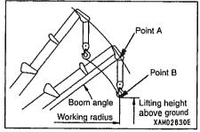
2. "Working radius/Lifting height Diagram" is bases on "no-load" without taking into consideration any bending of the boom.
