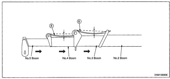
2. With the boom positioned horizontally and all the booms retracted, check to see if a clearance of 6mm or greater remains between the booms No.3 and No.4 (clearance (a)) and between No.4 and No.5 (clearance (b)). (See drawing to the right)
