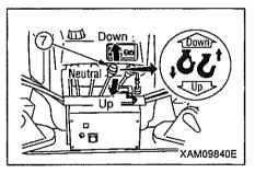
3. Disengage the hook block 4 from its hanger 3.
