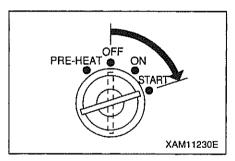
3. When the engine starts, release the key, It will return to ON position automatically.
