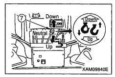
After that, push the winch lever 7 forward to Down position and lower the hook block.
