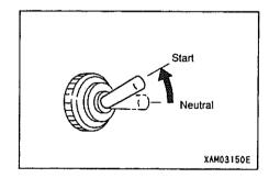
4. If the engine starts, release the auxiliary starter switch and the switch will return to Neutral position automatically.
