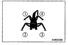
This machine has 4 outriggers. Method for setting up the outrigger is described below for the outrigger ③ only. The same applies to other 3 outriggers as well.
