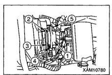
[2] Check oil level in travel motor reduction gear case, and add oil
