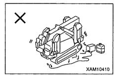
• Do not enter such place where temperature is high as bonfire, steel plate left in the blazing sun or newly paved asphalt.
