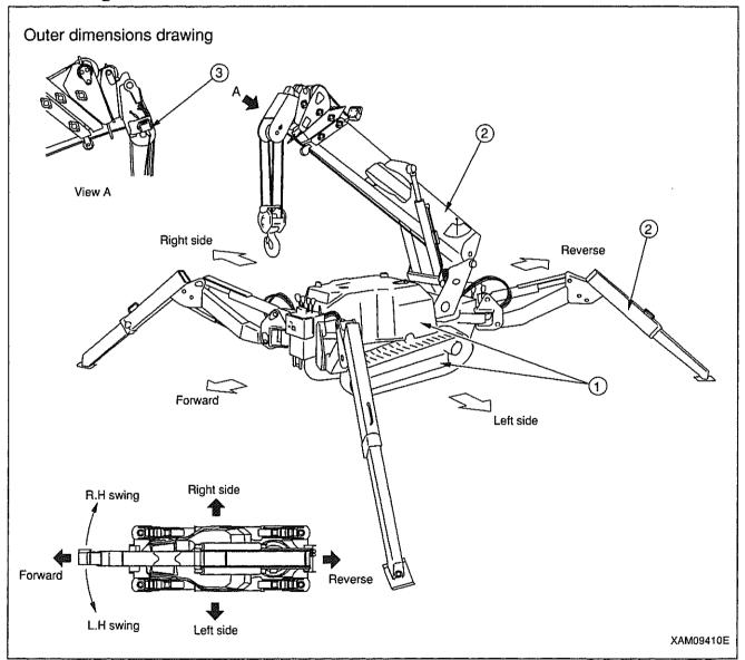
In this manual, front, rear, right and left are in principle identified respectively while viewing forward from the operator position. Above sketch shows the crane in working position.
