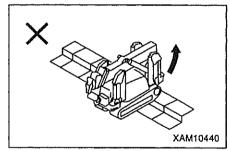
Rubber track becomes very slippery on any wet steel plate, snow covered or frozen road surface. Be careful about slipping during travel or work on slope.
