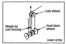
5. As shown to the right, thread the wire rope ⑤ through the fixed sheaves ⑩ and ⑪ at the end of boom No. 5.
