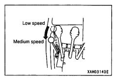
7. Slowly operate the boom hoist lever back and forth so that hoist cylinder extends and retracts to its stroke end to check that its function is normal. If not, correct it as necessary.
