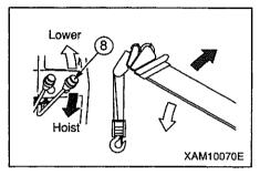
8. Slowly operate boom telescope cylinder back and forth so that the boom extends or retracts to its stroke end to check that its function is normal. If not, correct it as necessary.
