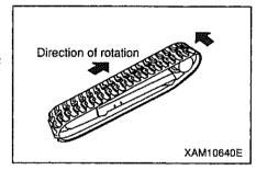
4. After inserting the steel pipe, rotate the sprocket again and engage the rubber crawler with the idler securely.
