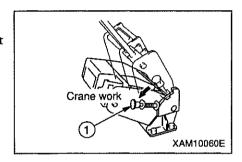
2. Place the winch lever ⑦ to Down position to loosen the wire rope which has been locking the hook block.
