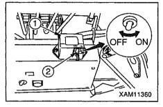
3. Press down the lever ④ of over-hoist alarm system ③ to check that the alarm buzzer stops.
