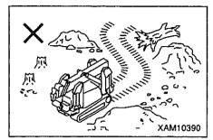
• At such job site as river location where great deal of boulders of various sizes are in existence, pebbles are likely to lodged and damage rubber track or to cause the track to come off.
