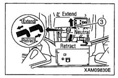
After that, pull back the boom telescoping lever e to Retract position and retract the boom.
