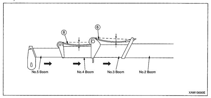
2. With the boom positioned horizontally and all the booms retracted, check to see if a clearance of 6mm or greater remains between the booms No.3 and No.4 (clearance ⓐ) and between No.4 and No.5 (clearance ⓑ). (See drawing to the right)
