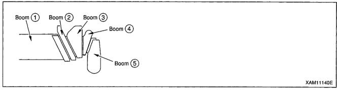
2. "4.075m Boom": With boom ② extended fully, remainder of booms are all retracted.
