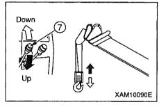
10. Slowly operate swing lever back and forth to check that the crane swings clockwise and counterclockwise smoothly more than 360 degrees respectively and that it stops immediately when the swing lever is returned to Neutral. Correct any abnormality as necessary.
