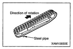
5. Stop the rotation and make sure that the rubber crawler is engaged with sprocket and idler securely.
