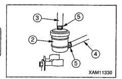
[3] Replace hydraulic oil return filter and suction filter
