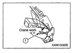
6. Pull back the accelerator lever on the crane control side to place the engine at medium speed (midway).
