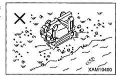
• Do not allow oil or chemical solvent to get on rubber track. Wipe it off. Do not travel over oil or the like gathered on road surface either.
