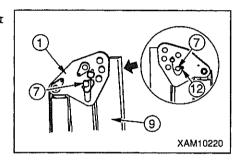
5. Lift up the top box <sup>(9)</sup> and align the hole of top box <sup>(9)</sup> with the position of the outermost hole on linkage bracket <sup>(1)</sup>.
